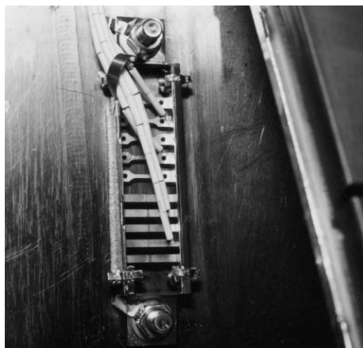
Fig. 2. Mounting of the W2 specimens in bracket on DIII-D vessel wall.
