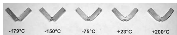
Fig. 4. Change of appearance of Charpy impact specimens with test temperature. The specimens are from the W2 test after \approx 4 -year exposure in DIII-D.
